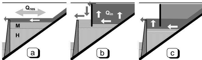
**Figure 1:** Schematic representations of flow-through regimes in the UWHA typical for summer stagnation periods before (a) and after the installation of the curtain (b: overflow over the curtain, c: underflow below the curtain).
