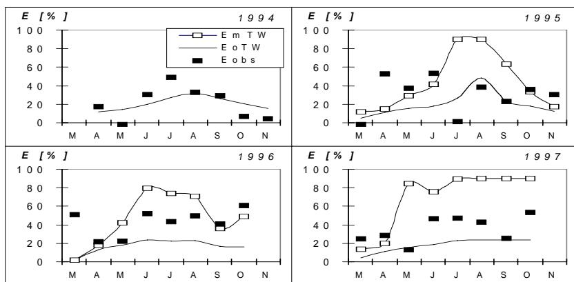
**Figure 2:** Observed SRP-elimination  $E_{obs}$  (determined with equation 2) compared with those estimated according to the procedure given by Benndorf and Pütz (1987a) assuming the SFC was not ( $E_{oTW}$ ) and was ( $E_{mTW}$ ) installed, respectively.
