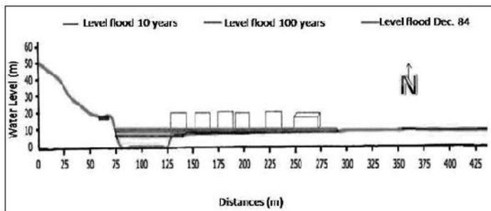
Figure 7: Wadi Saf-Saf in vicinity of the industrial zone: Cross section and levels of the probable peak flows
