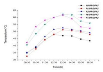
Figure 4: Evolution of the concrete temperatures as a function of time for different days
