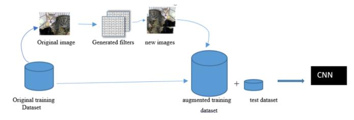
Fig. 1. Architecture of the proposed method used to generate augmented images.
